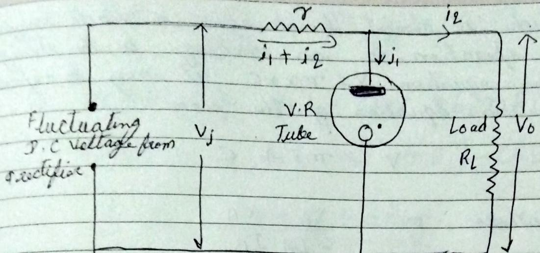
If the input voltage from the rectifier system increases, the voltage drop across the series resistor  $R$  increases and the voltage across the VR tube remains substantially constant.
