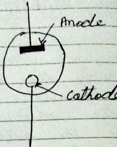
Due to cosmic radiation, some electrons and ions are always present in the gas. Ionization starts in the gas when a certain minimum potential is applied to the tube. Then a current flows through the tube the product of which with the internal resistance of the tube is equal to the voltage drop across the tube.
